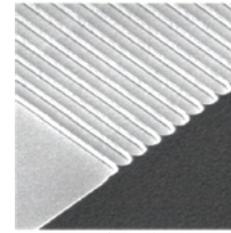
Figure 4: Tilt view SEM image of TaN metal lines – nano-wires – before planarization.
