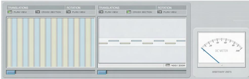
Figure 2: Idealised device showing strips of conductors in off-set position (top projection at left panel, cross section at middle panel, results in no current – right panel).
