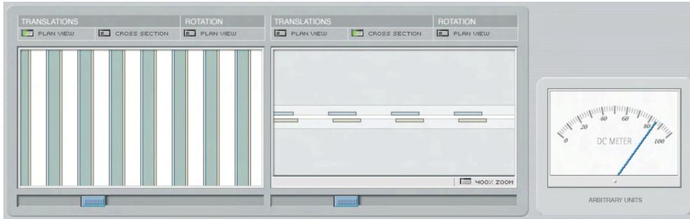
Figure 3: Idealised device showing strips of conductors overlapping each other (top projection at left panel, cross section at middle panel, max current – right panel).
