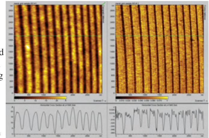
Figure 7. The AFM scans confirm SEM characterisation: well defined nanowires of width 90 nm are separated by 270 nm wide strips of insulator. The conducting nanowires are slightly below insulating strips surface, with 15 nm maximum variation in height. This experiment can in itself be considered almost a “realisation” of the Canon Patent “Encoder using the tunnel current effect” [4]
