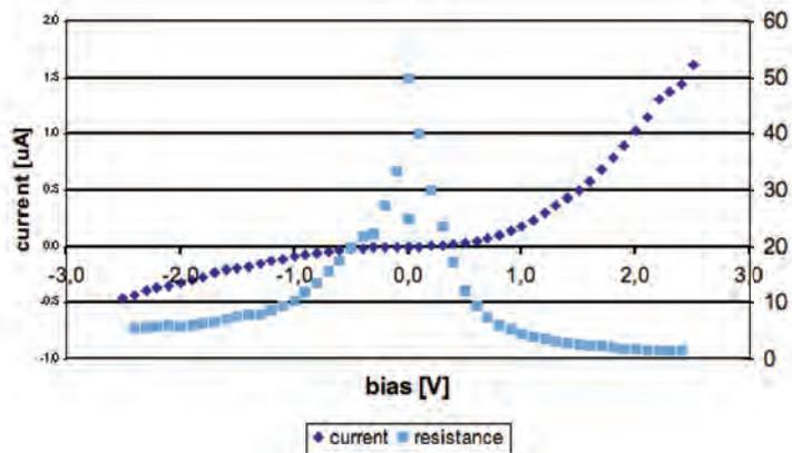
Figure 8. I-V characteristic of nanoTrek.
